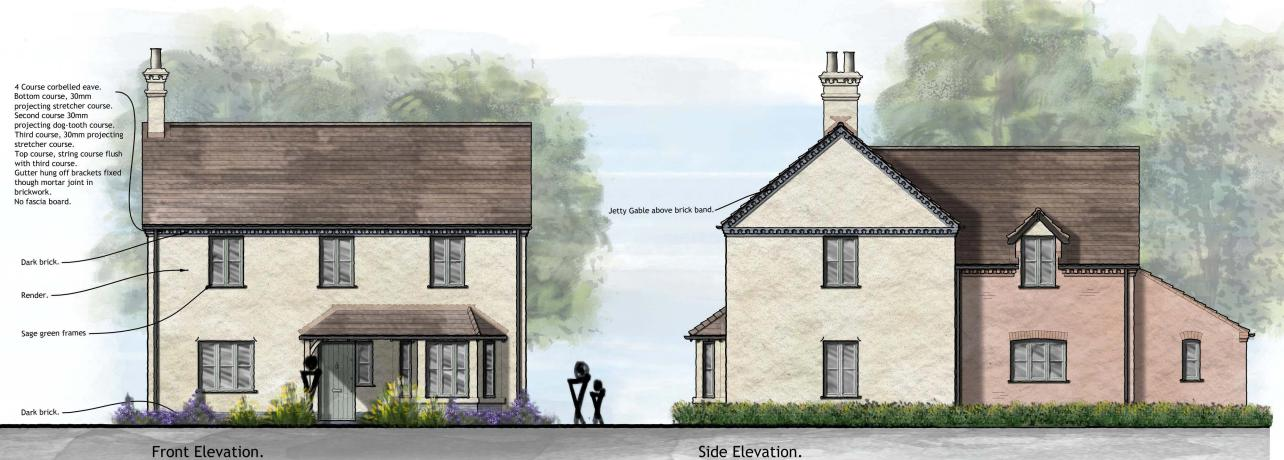
Dark brick courses and render to extend along the whole of elevation if elevation is exposed to the public realm.
