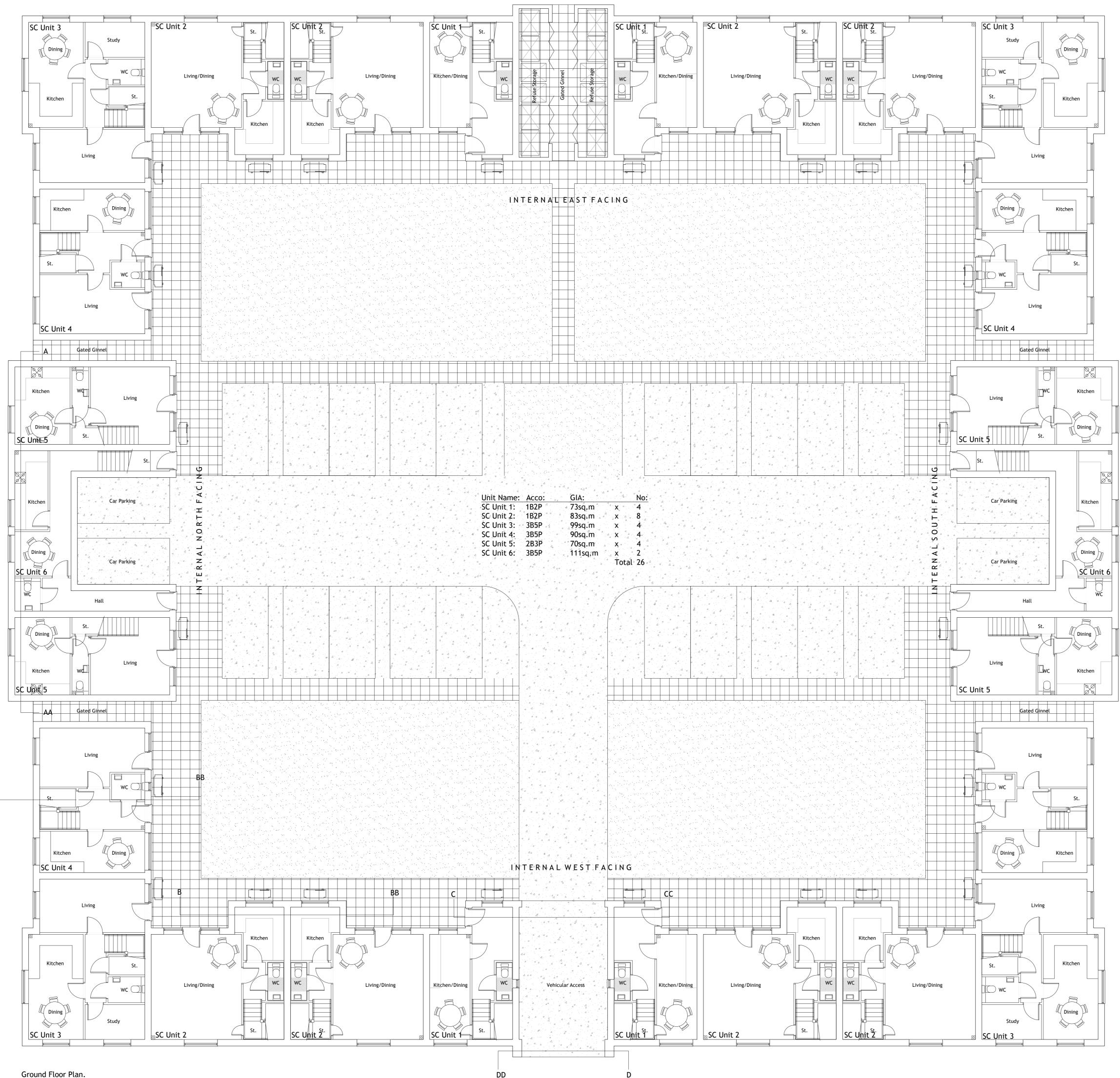
Ground Floor Plan. Stable Complex. M4(2) Compliant.
