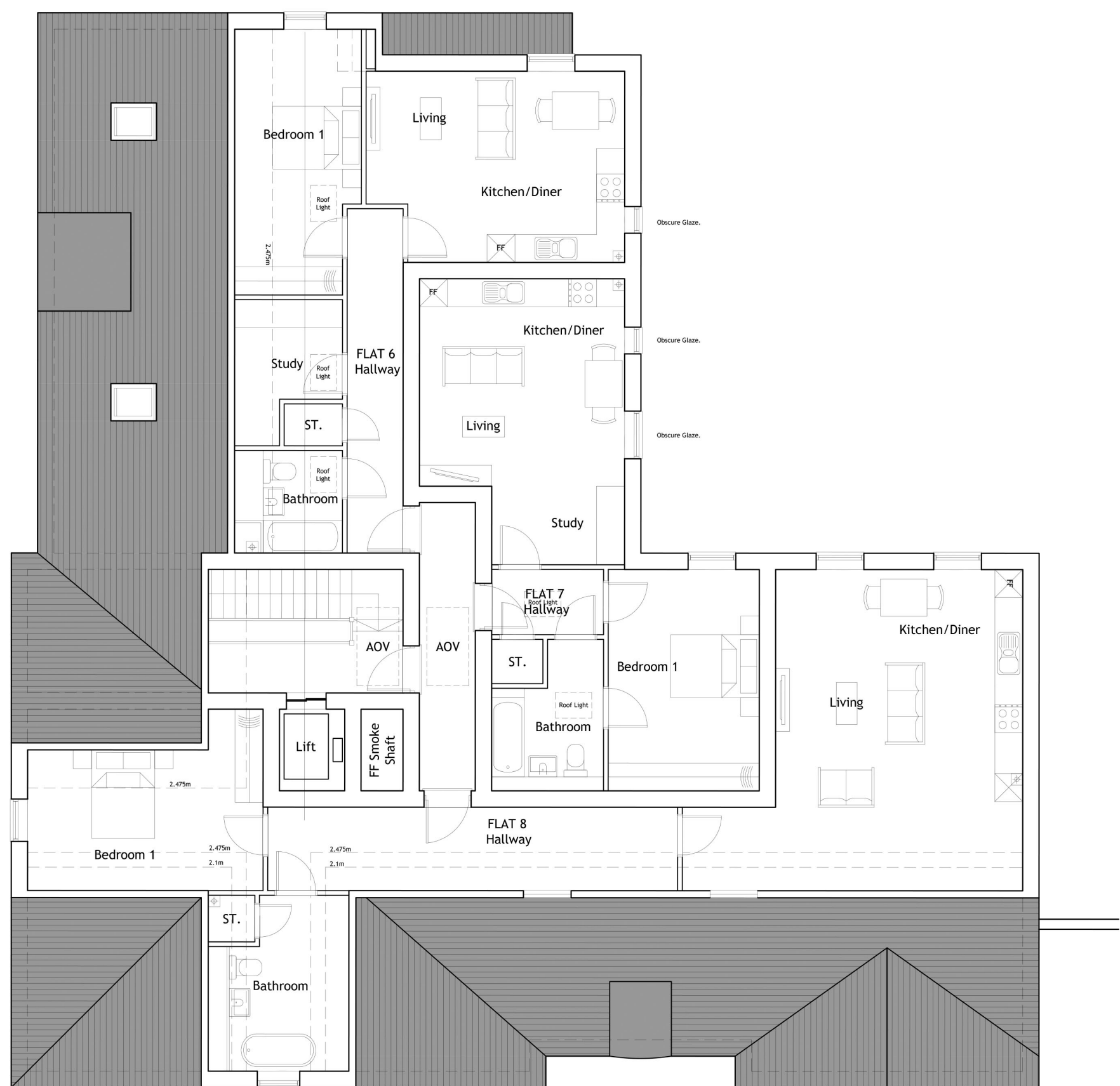
Second Floor Plan. Flats 6-8. M4(2) Compliant.
