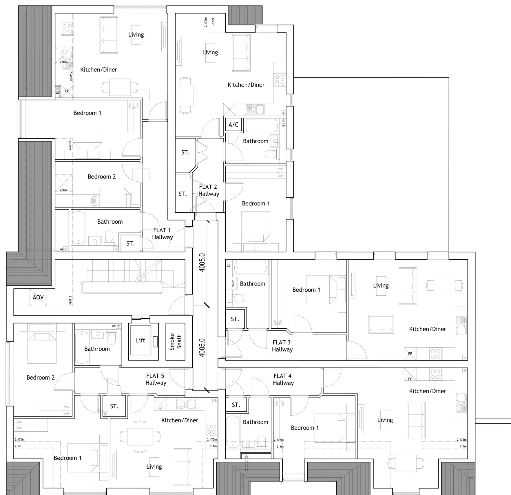
First Floor Plan. Flats 1-5. M4(2) Compliant.
