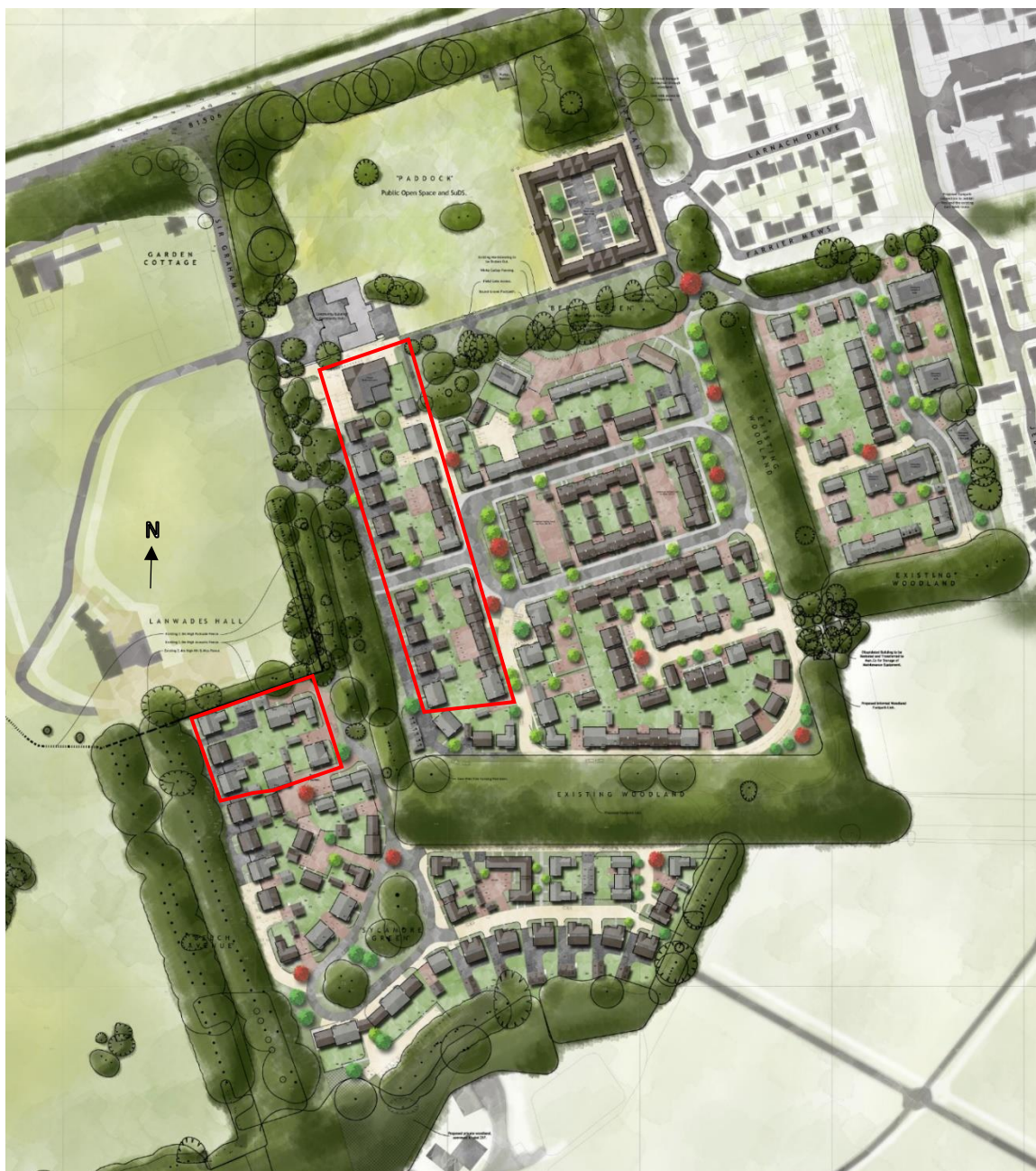
Figure 8.1 Residential units of the proposed development where a higher glazing rating (35 dB Rw+Ctr) is being proposed are encircled by a red line. The remaining units are proposed to have installed 29 dB Rw+Ctr glazing units. Detailed application – Red Line?
