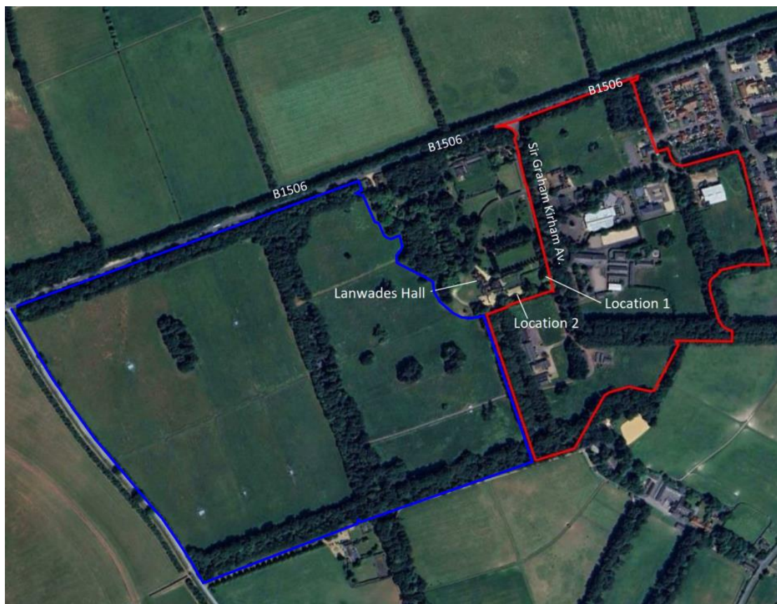
Figure 2.2 Location 1 and Location 2 (Condition 12 of Lanwades Hall Premises License) where music noise level should not exceed, respectively, 60 dB LAeq,15min and 65 dB LAeq,15min at any time during events. Boundary of the detailed and outline application is indicated, respectively, by a red line and by a blue line
