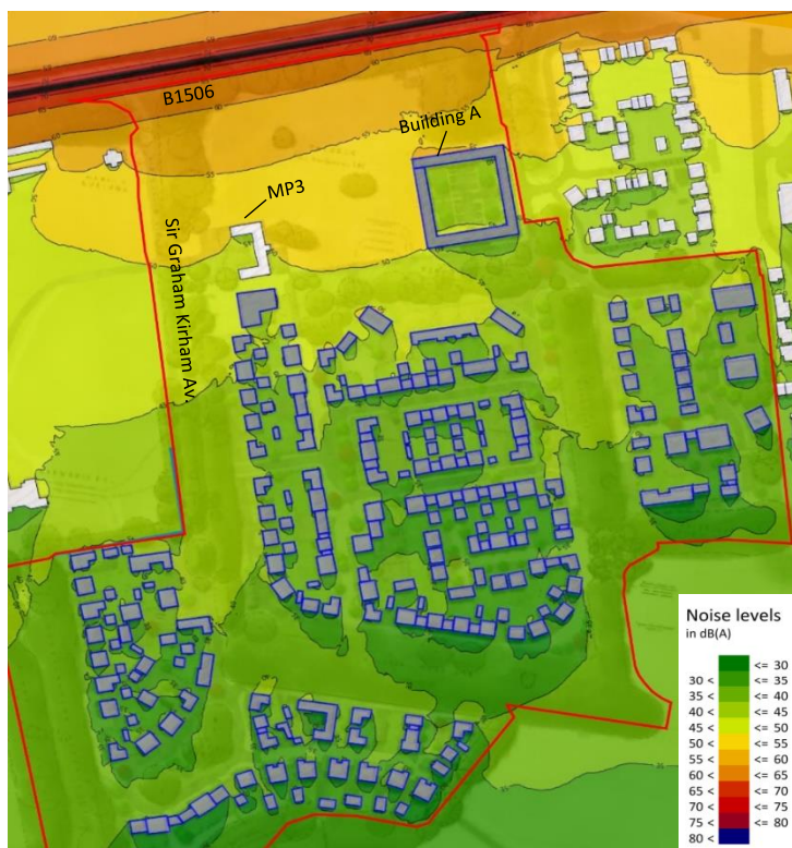
Figure 9.1: Day time traffic noise level predictions at the proposed development. Noise map at 1.5m height above ground level. The location of traffic noise survey, MP3 and of the residential building proposed to be built nearest to B1506, 'Building A' are also identified.
